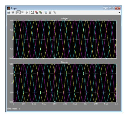
In this example, the **Component structure** parameter of the RLC block specifies that the electrical characteristics of the three-phase load are purely resistive. Therefore, for each phase of the three-phase system, the voltage and current remain in phase with each other. Because the resistance in each
