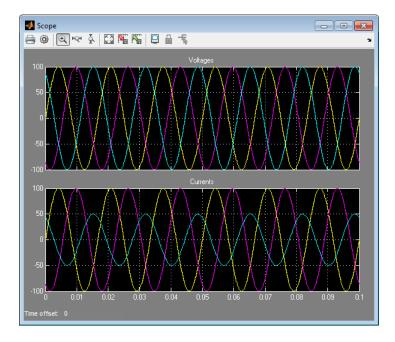
In this version of the model, one phase of the three-phase load has twice the resistance of the other two. Therefore, half as much current flows in that phase, as the second plot shows. However, because the load remains purely resistive, the voltage and current remain in phase with each other.
